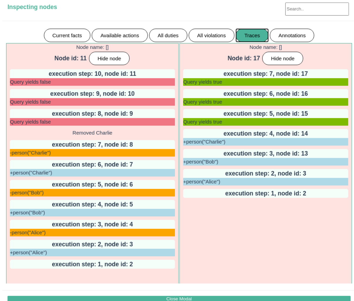
Figure 3.7: Comparing execution traces between different nodes in the eFLINT language. Each execution step can be clicked on to show more information, such as the code snippets that created the nodes.
